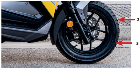
Recommended minimum tread depth: 2.0mm.
